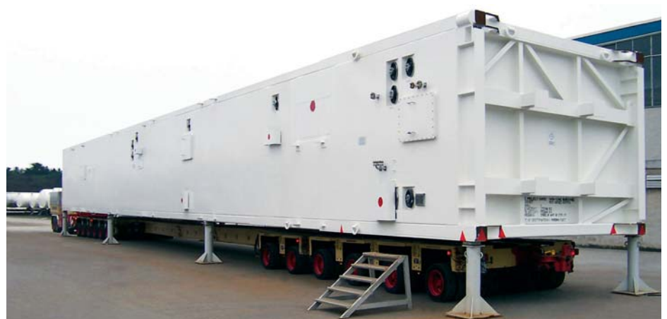
Packaged unit cold box
