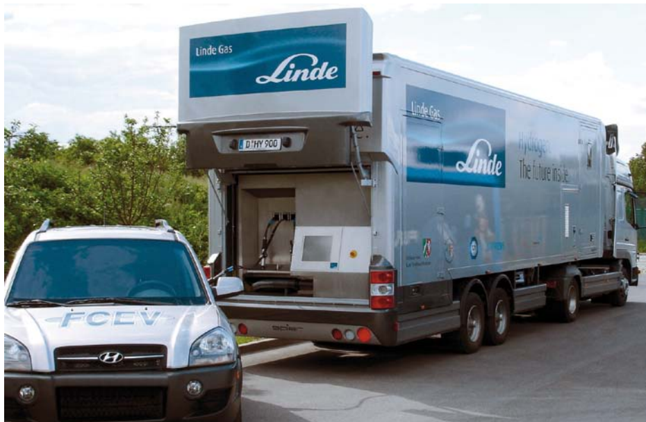
Mobile CGH 2 and LH 2 - fueling station
