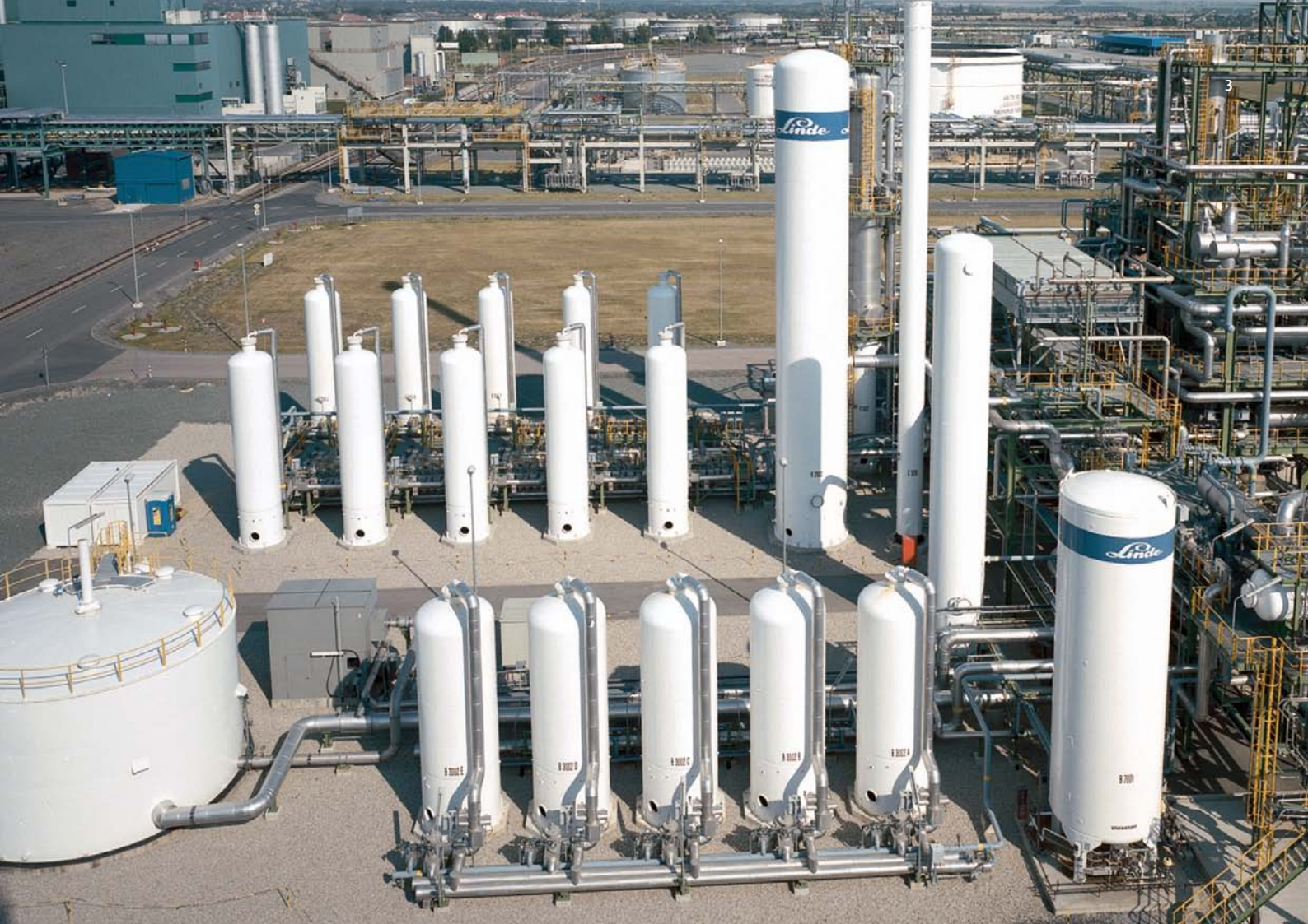
PSA units for H 2 and CO 2 recovery in a refinery in Germany
