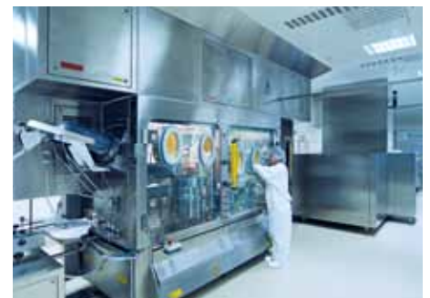
High-activity substances in a product isolator
