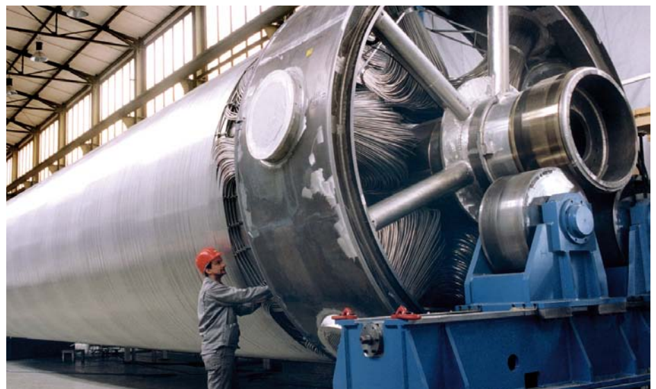
Coil-wound heat exchanger in Linde's own fabrication facility
