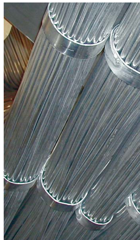
The tube bundles are designed and fabricated to be vibration-proof and self-draining.
