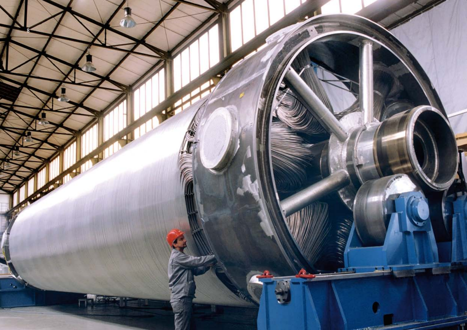
Tube bundle before insertion into the pressure vessel shell
