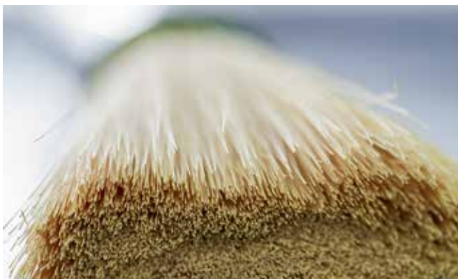
FIG. 1. Bundle of polyimide hollow fibers that will be woven into a membrane cartridge and packaged.
