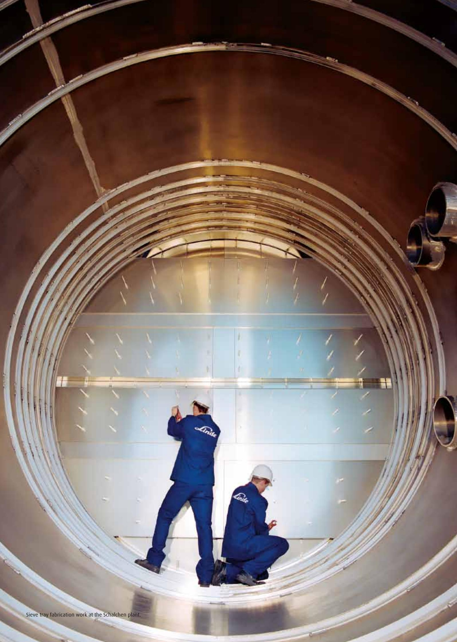
Sieve tray fabrication work at the Schalchen plant.
