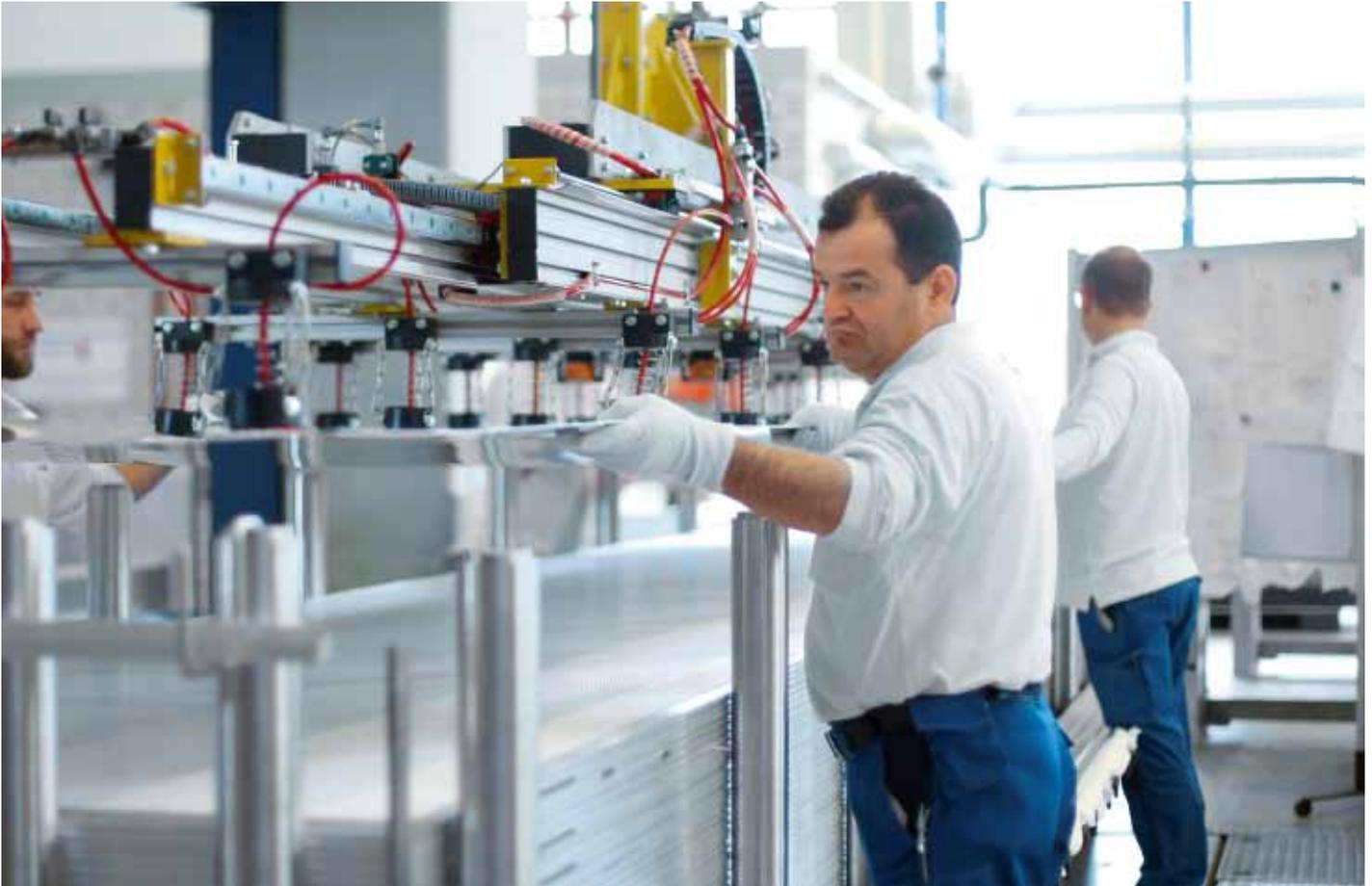
Aluminium plate-fin heat exchanger fabrication.
